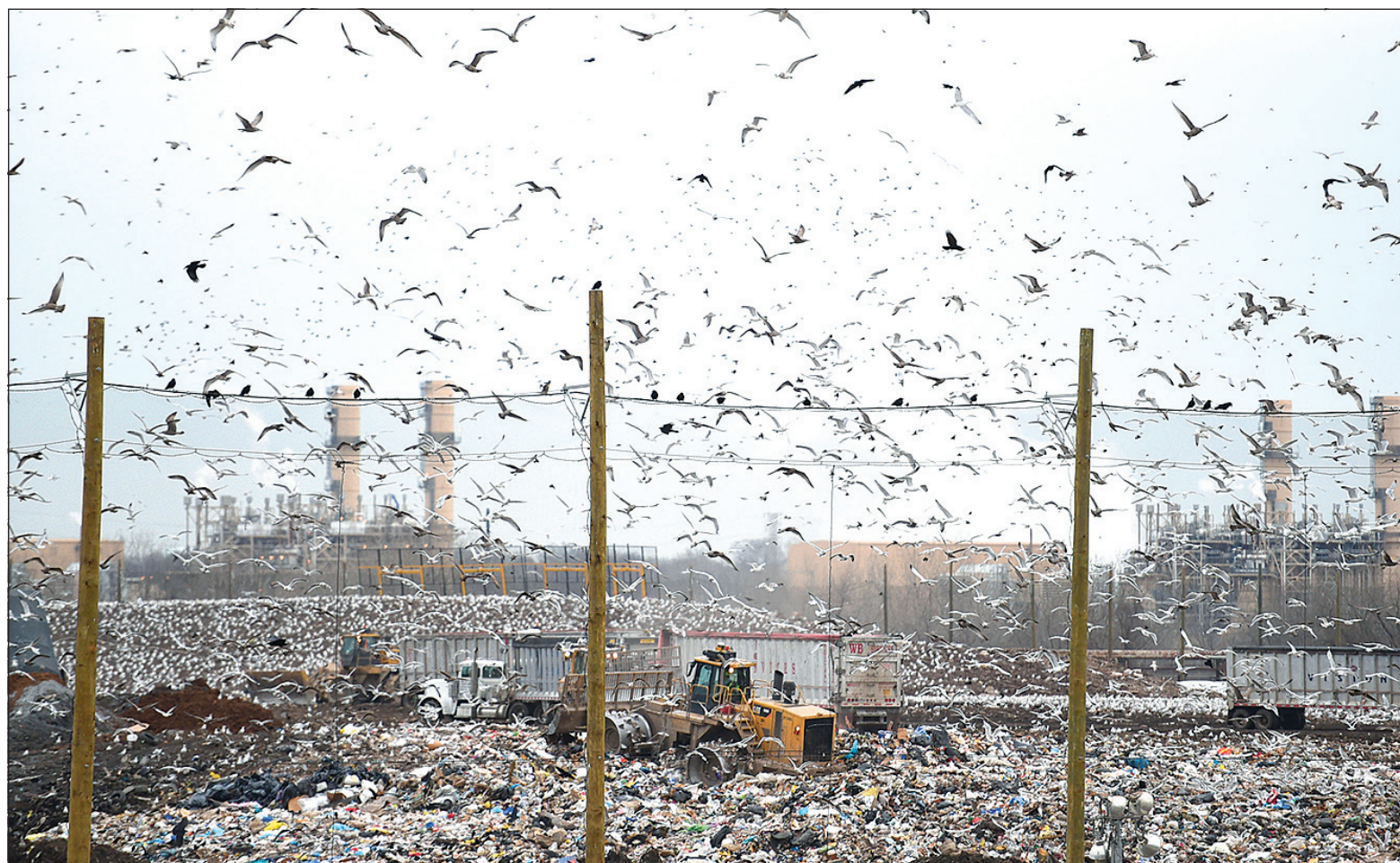
Bulldozers compact garbage at the Fairless Landfill at the Waste Management facility in Falls. CHLOE ELMER / PHOTOJOURNALIST
